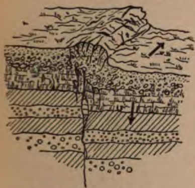
FIG. 61. — Diagram to show the appearance of a "mole hill" above a buried earthquake fault (after Kotó).
